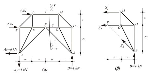
Passing the section  $\tau\tau$ , which intersects members 1, 2 and 3, we separate the right portion B $\Omega$ MOB (figure  $\beta$ ), which is under the act of the reaction B = 4 kN and the forces S<sub>1</sub>, S<sub>2</sub> and S<sub>3</sub>. Introducing all the unknown forces as tensile and writing the moment equation of equilibrium with respect to the point P, it yields:
