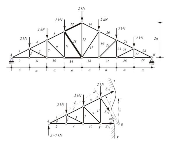
Drawing the free body diagram for the left portion, we notice that, before section, the portion  $A\Gamma\Delta$  of the truss was in equilibrium under the action of the known reaction A = 7 kN, the three vertical forces of 2 kN each, and, of course, those corresponding to the intersected members 12, 13 and 14.
