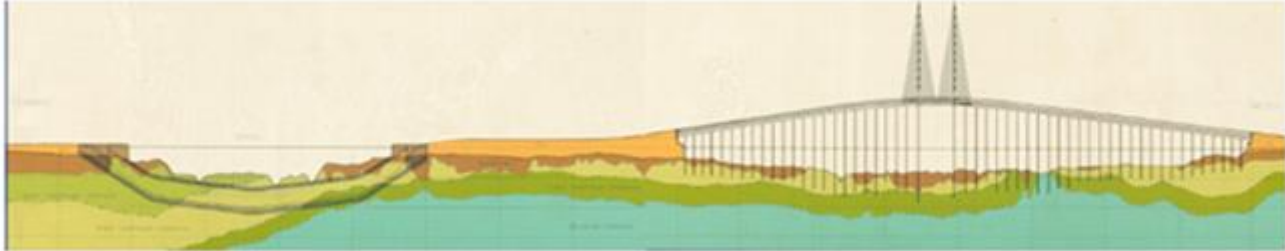
Fig. 5 A typical longwise profile from Copenhagen to Malmö in alignment (Light brown = fill, brown = glacial deposits & green, yellow, green = Upper, Middle and Lower Copenhagen limestone Units, blue = Bryozoan limestone) [18]
