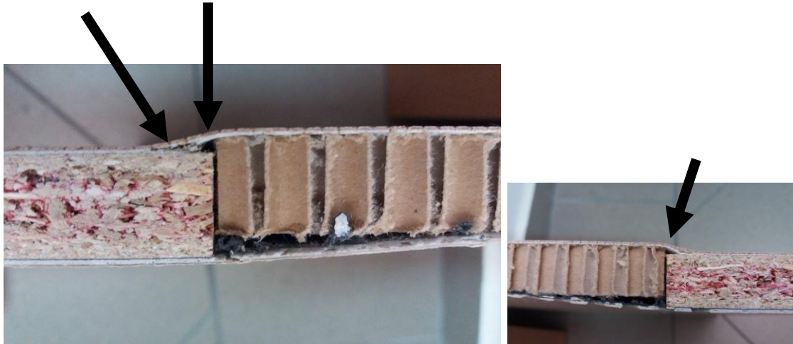
Photos 7a – 7b (photos taken by Dr. George Mantanis at the TEI of Thessaly) In the photos, it is very apparent the structural defects, right in the connection areas , that been taken place in the acoustic panels, i.e. defects very difficult to solve.
