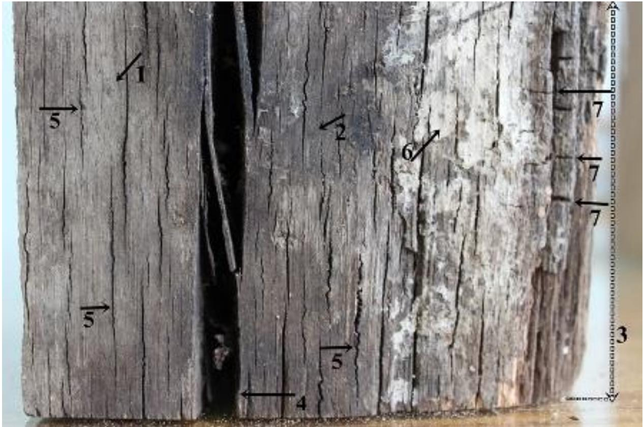
**Fig. 5.** Macroscopic view of the longitudinal surface of the old sample: Wood surface in silver gray (1) and darkish gray color (2), asymmetrical wood structure (3), splits (4) and checks (5) in the surface, a cottony white growth on the wood surface (6), and cubical cracks in the wood structure (7).
