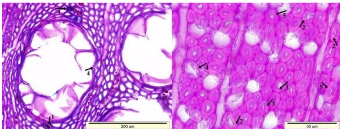
**Fig. 8.** Microscopic view of the cross-section of the heartwood sample: Dark colored residual materials in the lumen side of wood cells (1), clefts in the secondary walls of fiber cells (2), porous and swollen appearance in the fiber cell walls (3), distortion in the shape of the wood cells (4), and a much more degraded S<sub>2</sub> layer of fiber cell walls (5)
