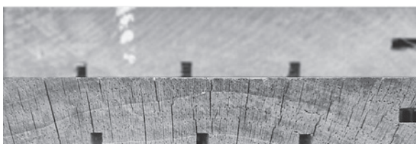
Figure 13 Furfurylated radiata pine wood deck prior to (up) and after 36 months of weathering (down)
