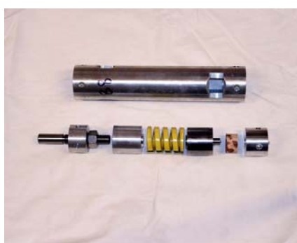
Figure 4.2.6: Creep-rupture testing device. (Figure from Bengtsson and Johansson 2001.)
