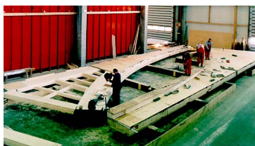
Figure 4.4.5: The assembly of the box-beams of girder. The flanges are made of glulam and two Kerto-Q boards thickness of 33 mm are screw glued both sides of flanges. The upper flange is straight and the lower one is curved
